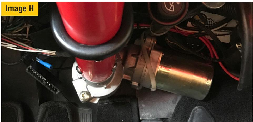
Install the pre-wired control module on the firewall just next to the fuse block (or elsewhere), hook up the power wire for the motor (blue connector) and the connector for the torque sensor (Delco weather-pack). Then hook up the small red wire to a hot in run and the #10 red wire directly to your battery or a direct power source. You can use a 60A fuse if desired.
